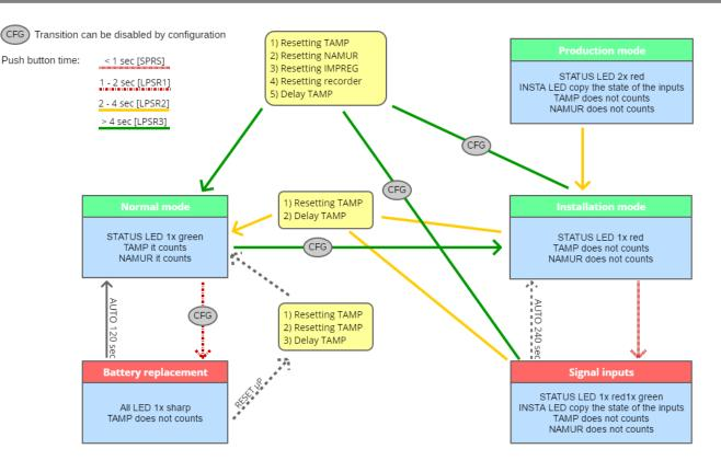
Before installing, remove the top cover of the module to get to the terminal board and the MENU control button. The installation should always take place when the module is in the installation mode. In the installation mode, the module is shipped from the manufacturer. We recognize the module mode by flashing the two-color status LED. If the module is in normal mode, it is necessary to switch it to the installation mode by long press of type 3 MENU button.
