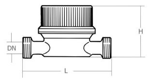
• for DN15 and DN20 height H = 63 mm
